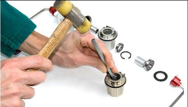
A photograph showing a person's hands performing a repair. The person is wearing a green sleeve. They are using a hammer with a yellow head and a wooden handle to strike a metal punch. The punch is being used to drive a bearing out of a cylindrical metal housing. The housing is held steady by the other hand. To the right, the disassembled components from the previous image are visible, including the metal cage, rings, and O-ring. |
