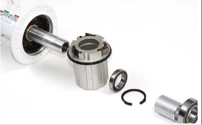
A close-up photograph of a disassembled free wheel mechanism. The main component is a cylindrical metal housing with a central shaft. To its right, the internal components are laid out: a cylindrical metal cage, a small metal ring, a black O-ring, and another cylindrical metal part. The background is white.                                                                                                                               |
